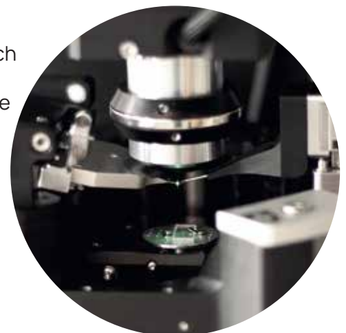
Probe and near-field antenna, with sample retracted
