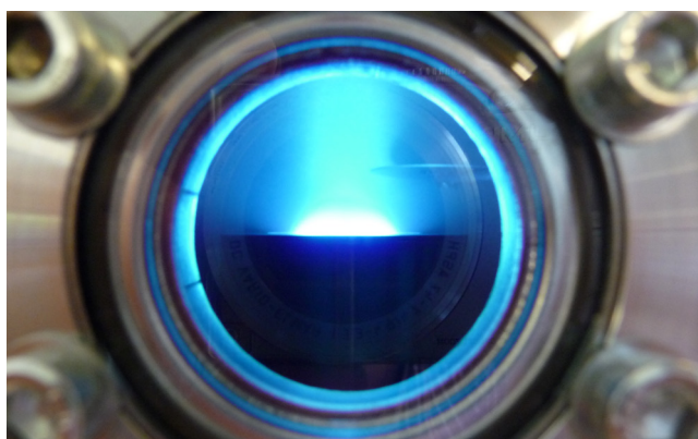
View through chamber viewport, showing operating magnetron sputtering source on nanoPVD-S10A
