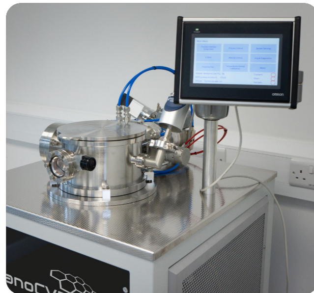
High vacuum chamber, HMI, and pumping system to the rear.
