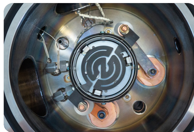
Chamber with lid opened to reveal inner components and heat shielding. The capacitance manometer and wide-range gauge for pressure measurement are visible to the right of the chamber.
