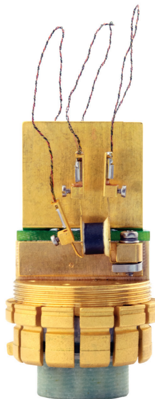
TTO Puck with Disk-Shaped Sample Installed
