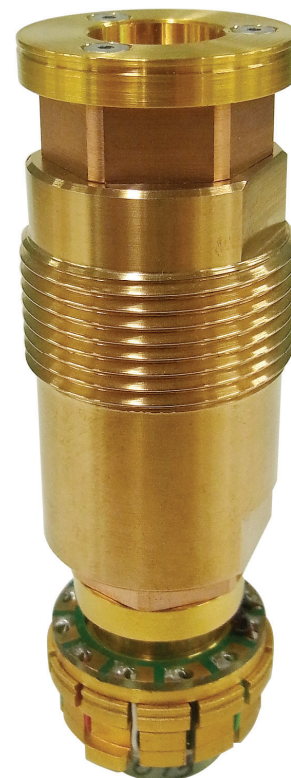
High Pressure Cell for Electric Transport Measurements
